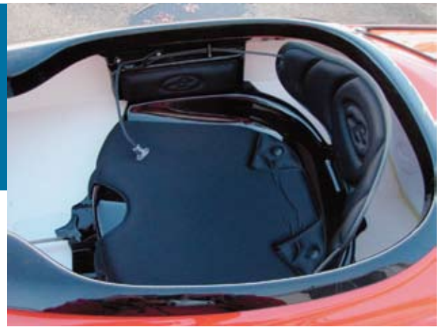
The knob at the front of the seat allows you to adjust the fore-and-aft position of the seat.
